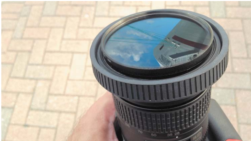
FIGURE 6.21 The use of a neutral density (ND) filter can really cut down on exposure problems when shooting outdoors.
