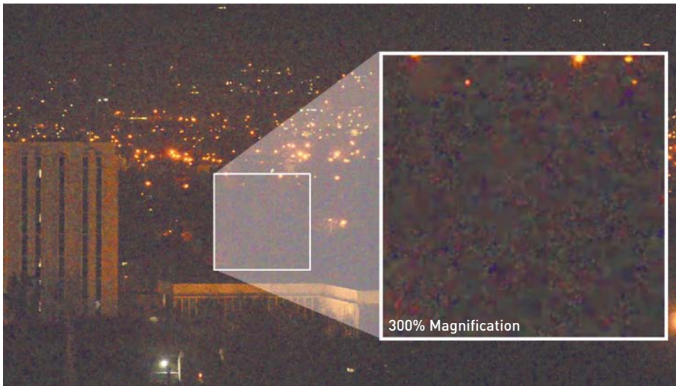
FIGURE 4.5 The noise becomes very visible in this low-light image. In this case, an ISO of 6400 was used; however, it produces an unusable image. Be careful not to boost your ISO too high when shooting in low light, or visible noise will ruin the shot.
