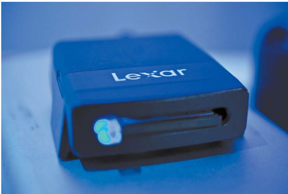
FIGURE 10.2 A fast card reader will speed up the transfer of your footage. This device from Lexar connects to your computer via a FireWire 800 connection. Photo by Lisa Robinson.
