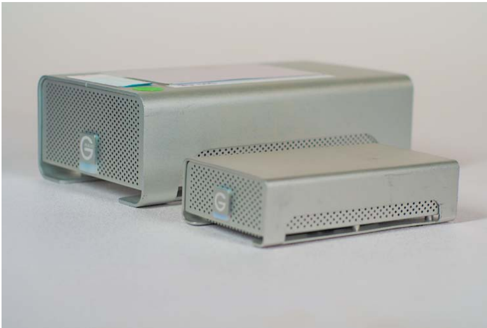
FIGURE 10.4 Both of these drives offer RAID 0 performance: One is a desktop drive, and the other is meant to be portable for laptop use. RAID 0 means that two drives are in each case and split data evenly across the two disks (referred to as striped ) to work more efficiently for the higher data throughput demands of video editing.
