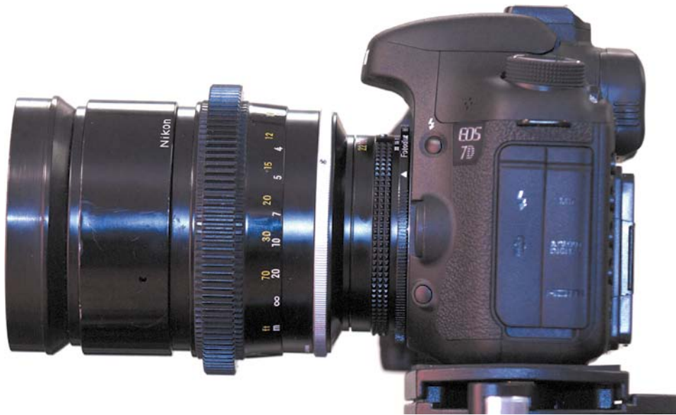
FIGURE 4.11 An older Nikon prime lens is attached to a newer Canon 7D using an adapter ring from Fotodiox. Lenses need manual aperture and focus rings to work properly with the adapters.
