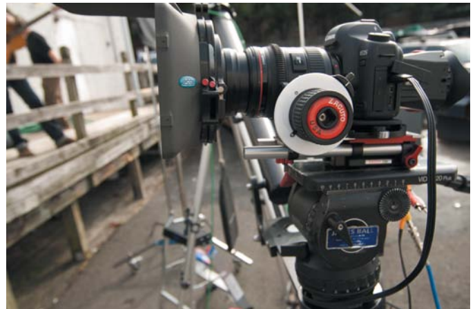
FIGURE 1.12 This DSLR camera has been converted to a film-style camera. Equipment like a matter box (for adding filters to the lens) and a follow focus (to make it easier to focus on a moving subject) complete this pro-style camera package.
