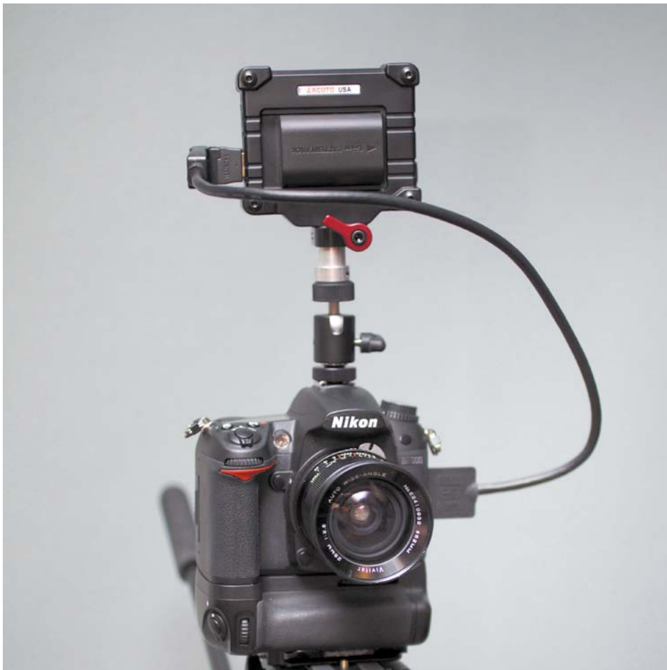
FIGURE 4.14 The Zacuto Electronic Viewfinder, combined with Zacuto's loupe, creates a complete monitoring solution.
